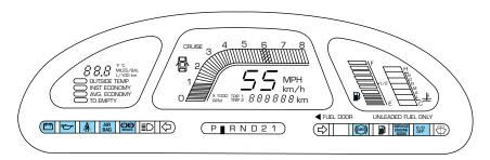
Make sure the corresponding lights illuminate briefly. If a light fails to illuminate, have the vehicle serviced.
